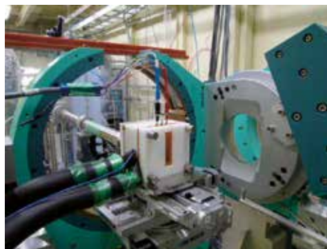
Fig. 8 Developed Temperature-Controlling Tool for Synchrotron Radiation Diffraction
