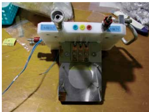
Fig. 2 Developed Temperature-Controlling Tool for Neutron Diffraction
